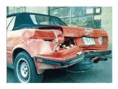
The middle steel guard rail cable had sliced through the trunk, while the upper cable had slid up over the trunk lid and sliced into the back of the convertible top, just a few inches from our necks. The front of the car suffered similar triple gashes.
